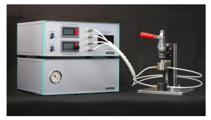
The upper display (optional) of the mass-flow-meter should be at the same value with a maximum deviation of 0.2 l/min. If the shown value is out of range more than 0.2 l/min, the inserted material must be checked for creases and the sample-holder for correct closure.
