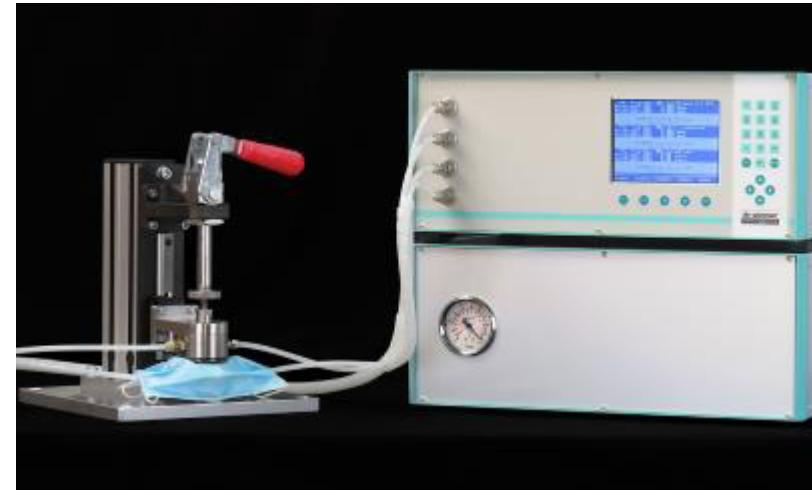
Channel 1 is used for adjustment and counter measurement of the flow rate, according to internal test guidelines.
