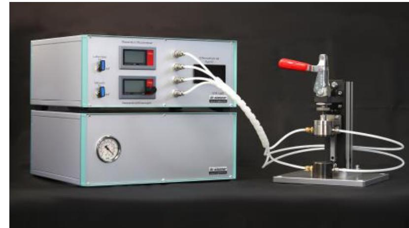
The upper display (optional) of the mass-flow-meter should be at the same value with a maximum deviation of 0.2 l/min. If the shown value is out of range more than 0.2 l/min, the inserted material must be checked for creases and the sample-holder for correct closure.
